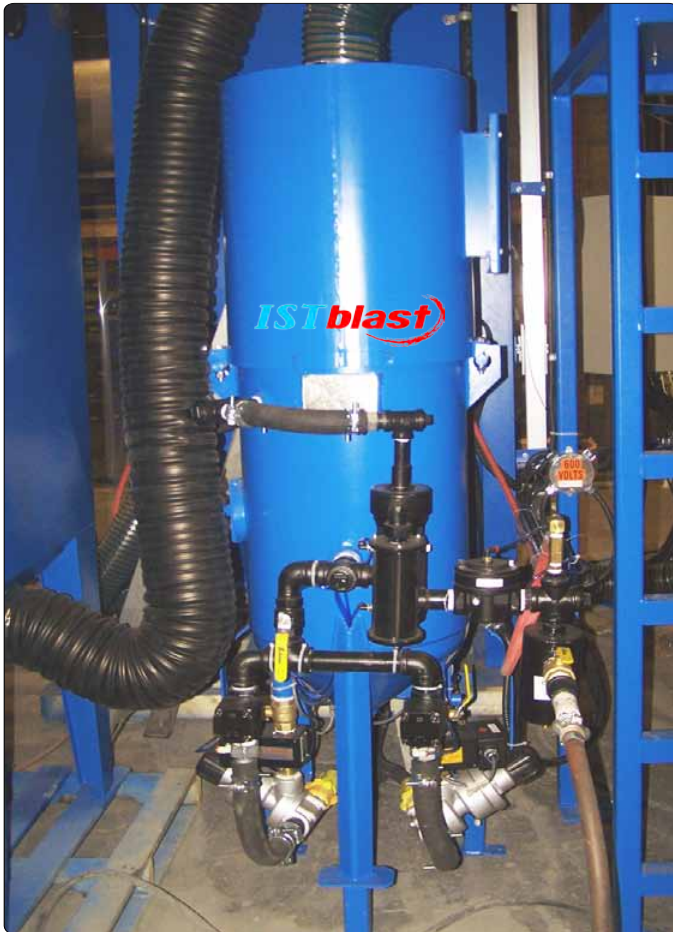
Model 646 6.5 ft 3 capacity With Magna valves
