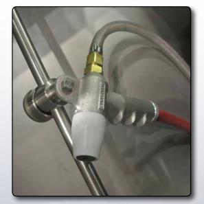
A G5-BN2-5 suction gun (see parts ass'y p. 15) with a wetblast type head equipped with a boron carbide nozzle is mounted on an adjustable arm.
