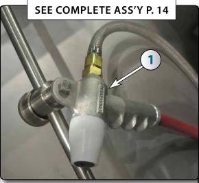
A G5-BN2-5 suction gun (1) with a wet-blast type head equipped with a boron carbide nozzle is mounted on an adjustable arm. The blow-off gun (6) allows the part being blasted to be cleaned and free of the mixture of abrasive/water.
