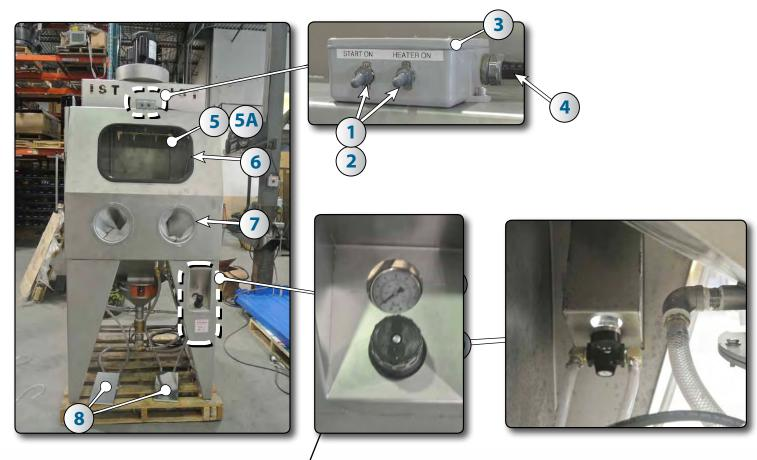
With a suction system such as this one, for the highest blasting performance it is recommended not to exceed a pressure of 80 psi.
