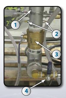
If the machine is stopped for more them 2 days and to prevent the formation of a plug between the reservoir base (1) and the superior part of the valve drain (3), 2 solutions are proposed:
