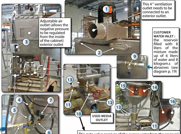
This gate-valve receives all the excess water from the reservoir and the gutter. It is recommended that the main drain be connected to an evacuation drain and that the gate-valve stay open. The evacuation drain (12) allows the mixture to be emptied after a certain period of machine use.
