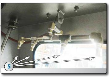
The interior of the window is equipped with a window washer system activated by a pedal. The pneumatic diagram of this system is shown page 17.
