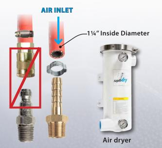
**Connect your shop's air supply line to the air inlet.** The hose should have a minimum of  $\frac{1}{2}$ " inside diameter. Never use male-female quick couplings. **Choose couplings that offer as little restriction to the airflow as possible.**
