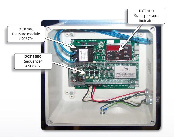
Sequential controller DCT-1000 dust collector used in conjunction with pressure module DCP 100 Their operation is described in the documents attached pages 46 to 48.
