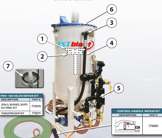
Note: Refer to owner's manual for complete part list of the pressure vessel. Address maintenance procedure to any air leaks occurring in between the schedule maintenance.
