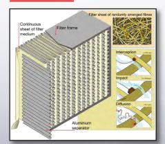
Our standard reverse pulse cartridge dust collectors trap 99.7 percent of dust particles as small as 0.5 microns. A High Efficiency Particulate Air (HEPA) filter captures 99.97 percent of the remaining dust particles (down to 0.3 microns).
