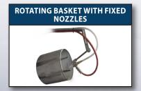
The combination of the basket inclination, rotation speed and time of exposition to media flow can speed up an increase blasting quality of batches of small parts.
