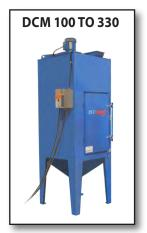
Inside the dust collector, a dry filter contains a set of cotton sating tubes that act as a filter for exhausting clean air flow from cabinet. Periodically, the clogged filters must be shaken to knock the dust from the insides of the tubes into a tray at the bottom of the dust collector. From time to time, the operator must empty the tray.
