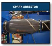
Mounted on dust hose linking the media reclaimer to the dust collector in order to eliminate the risk of fire
