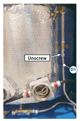
**4.** Unscrew the the flexible hose **[D1]** and lower it to an oil pan in order to remove oil inside it, then tighten it in place.
