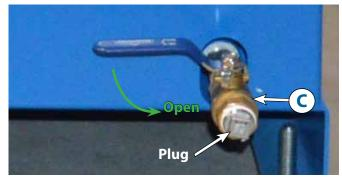
Remove the plug and drain oil out of the oil cooler tank by opening the ball valve [C] after placing an oil recuperation pan below or connect it to a pump.
