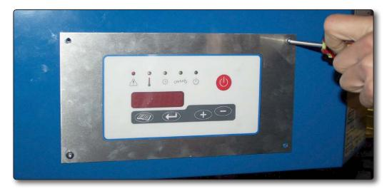
2. Delicately remove the plate from the front of the machine.
