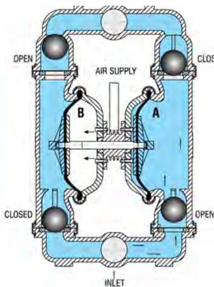
The air-valve directs pressurized air behind the left diaphragm, causing the left diaphragm to move outward (to the left).
