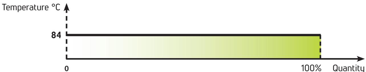
The distillation temperature of a clean solvent remains the same until the process of the whole cycle is complete.
