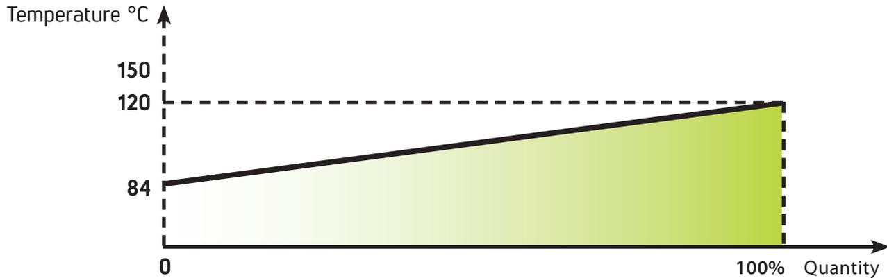
Operating with vacuum condition, 100% of perchloroethylene will be recovered when set at 120°C (248°F) and very far from the critical temperature of 150°C (302°F).
