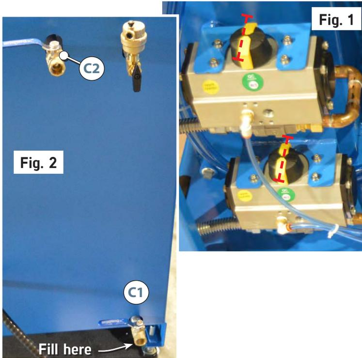
Before you begin, ensure the 2 Rotex valves (Fig. 1) are closed.
