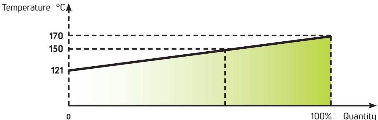
Once a temperature of 150°C (302°F) is reached, which is the critical non-supportable temperature, only 80% of perchloroethylene will be recovered.
