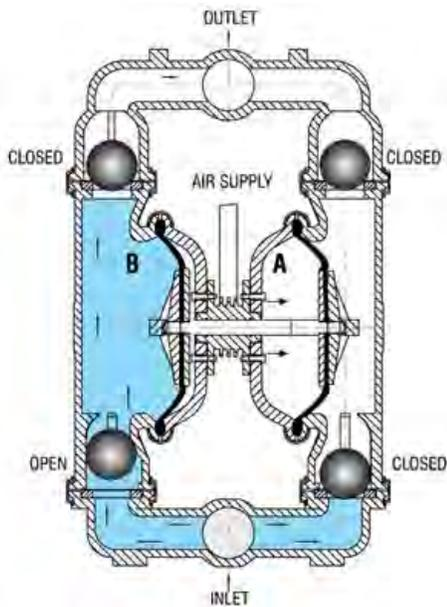
The air-valve directs pressurized air behind the diaphragm on the right, causing the diaphragm on the right to move outward (to the right).
