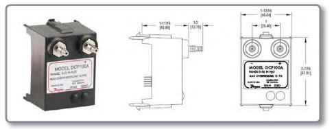
The DCP100A or DCP200A pressure modules are designed exclusively for use with the Dwyer DCT1000 Dust Collector Timer Controller boards for on-demand cleaning requirements. These series of modules are available in 10" w.c. [2.49 kPa] or 20"w.c. [4.98 kPa] ranges, which allow for differential process pressure measurement as indicated on the display of the master controller. An isolated 4-20 mA readout channel is
