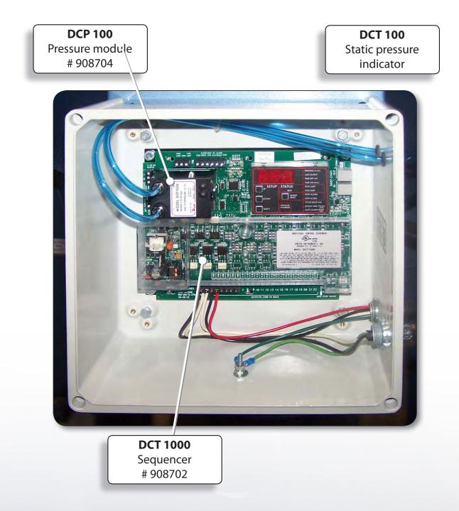
Sequential controller DCT-1000 dust collector used in conjunction with pressure module DCP 100 Their operation is described in the documents attached pages 46 to 48.
