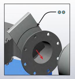
It should be bolted directly to the output of the fan located on the dust collector. Make sure the exhaust gate valve is between the fan and the muffler. If required, adjust the gate valve to the <u>black mark</u> on the housing.
