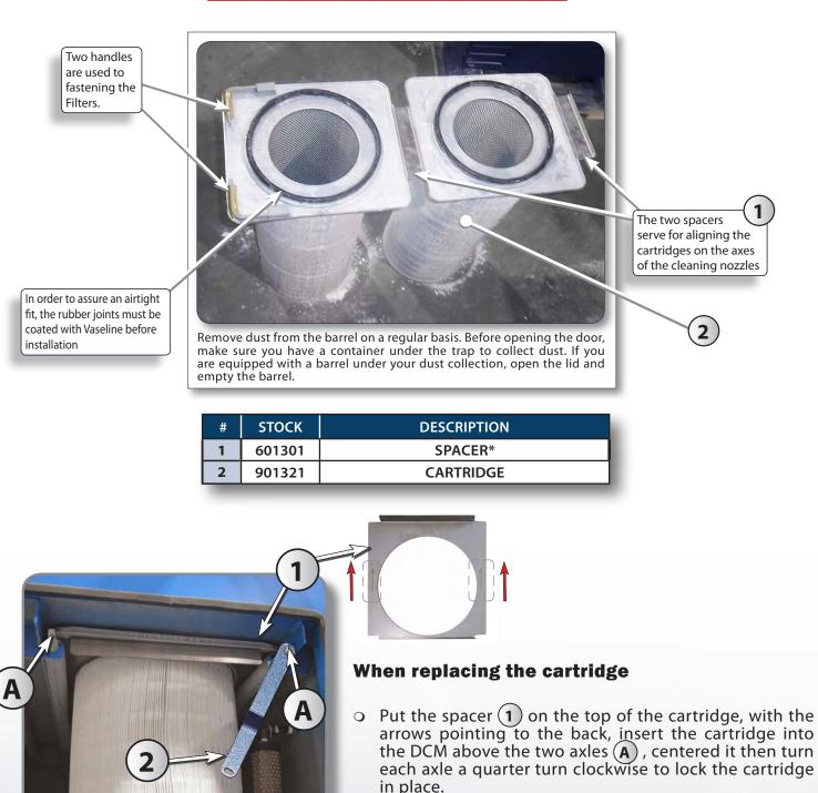
• Repeat the same operation with the cartridge 2, 3 and 4 if necessary.
