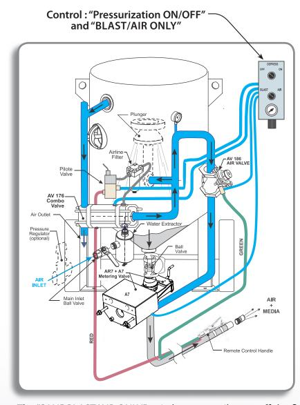
The air line feeds air to an AV-176 Combination Air Intake and Exhaust Valve, which is usually closed.
