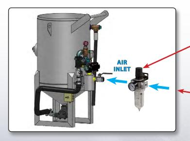
Install a 1¼ "air regulator (not included) to stabilize the internal pressure in the pressure vessel and in the sandblasting hose.
