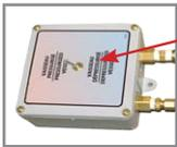
5. Pressurize the pressure vessel with the control unit by turning the switch to **"PRESSURIZED VESSEL"**. The vessel should pressurize at the blasting pressure already preset.
