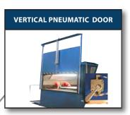
Vertical pneumatic door allows for wider openings and reduced footprint.
