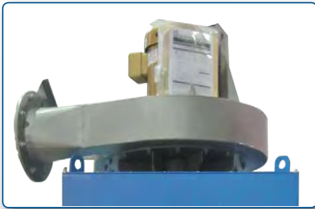
Impeller extraction system 10 hp / 800 cfm for MRS200
