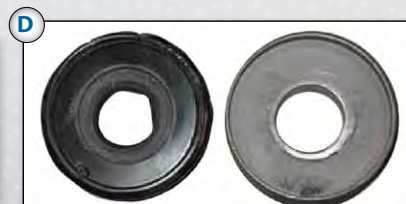
Urethane Seat (left) is completely intact with normal wear. Stainless Steel Insert (right) shows no signs of wear.
