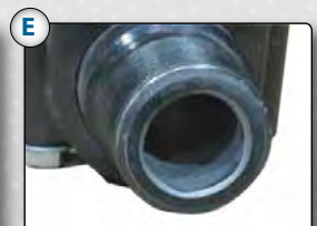
Metering Valve Nipple 1½ shows only minimal wear.
