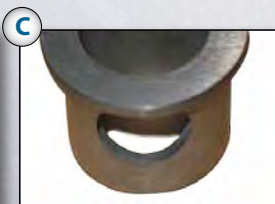
Only minimal signs of wear showing on sleeve.
