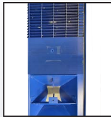
Pneumatic recovery system with floor hoppers
