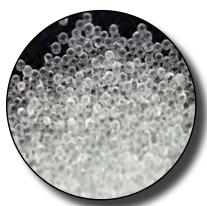
Glass Bead is one of the most popular abrasives used in cabinets today. Chemically inert, it produces a clean surface for parts and equipment without deteriorating the surface due to its moderate aggressively. Glass Bead is also environmentally friendly and can be disposed of at low cost, without extensive paperwork
