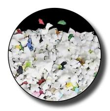
Plastic Media is a dust-free abrasive produced from special alloy of plastic material that has high tensile, compression, and flexural strength combined with comparatively low hardness. It is gentle on workpiece surface, but very effective for cleaning or removing paint, coating, and other stubborn materials.
