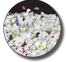
Plastic Media is a dust-free abrasive produced from special alloy of plastic material that has high tensile, compression, and flexural strength combined with comparatively low hardness. It is gentle on workpiece surface, but very effective for cleaning or removing paint, coating, and other stubborn materials.
