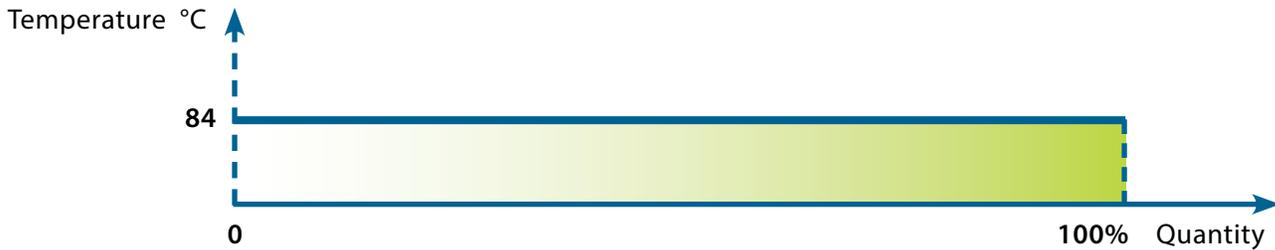
**C.** Boiling range at atmospheric pressure (1,000 hPa) of a mixture of 90% perchloroethylene + 10% of oil.
