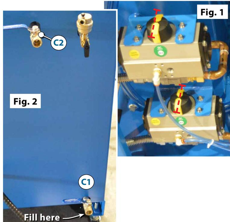
Remove the plug, and connect here. (the 2 boiler ball-valves **must be in open position**, but the 2 cooling tank ball valve **must be closed** to avoid over filling it)
