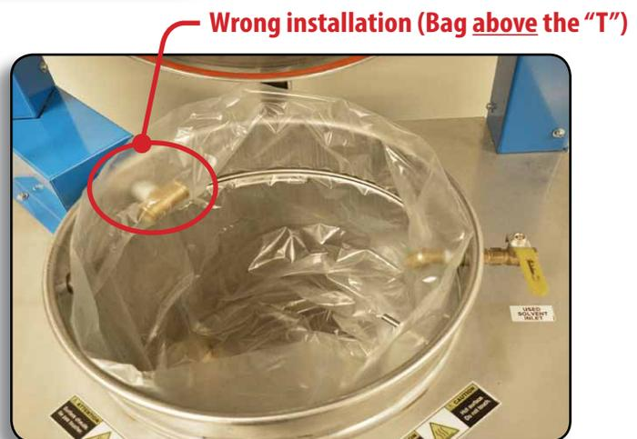
**Note :** the recycler boiler shown above is a SR30, but the principle is the same for all models.
