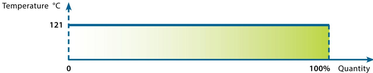
**B.** Boiling range of clean perchloroethylene at vacuum condition: 223 hPa
