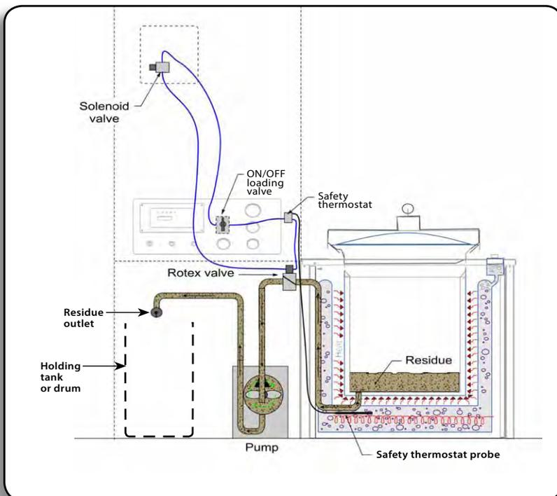
The standard sludge discharge feature is manually done by the operator. Upon completion of the process and once the sludge is below 75° C the operator will position turn the un loading valve to the on position to activate an air Operated Diaphragm Pump. If the temperature is above 75° C the pump will not be activated because it is protected by a safety thermostat.
