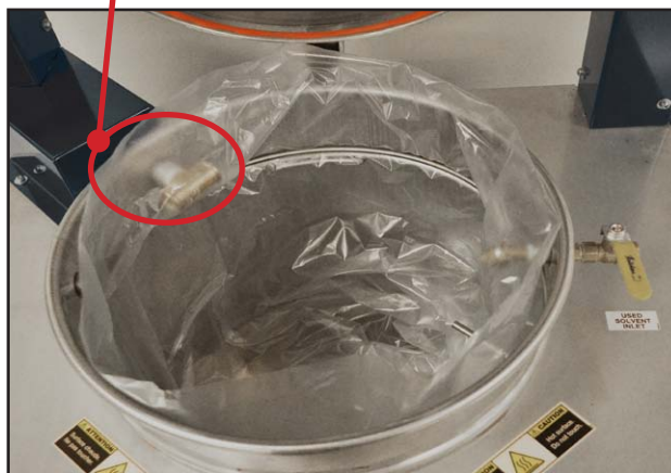
Wrong installation (Bag above the elbow)
