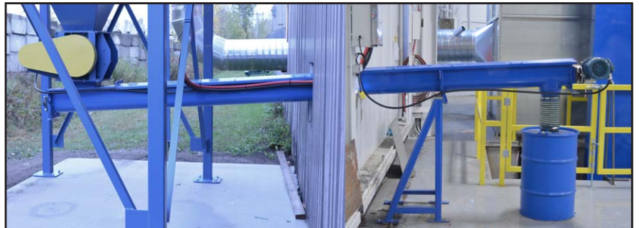
Optional screw conveyor to collect dust inside the building
