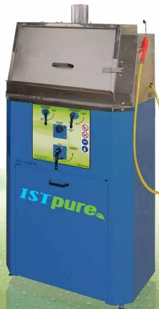
ISTpure's spray gun cleaner GWMA 500 is an ergonomic and robust cleaner that is suitable for medium-to-heavy users with repetitive color or coating changes. Its combined manual and automatic cleaning station allows to clean efficiently up to two paint spray guns along with PPS and other disposable cup adapters simultaneously in less than 30 seconds using the automatic wash setup or to proceed to a full-wash of disassembled guns using its manual wssh setup and tools.
