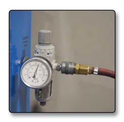
We strongly recommend using a dirt / water trap and an air pressure regulator when using your GWMA700.
