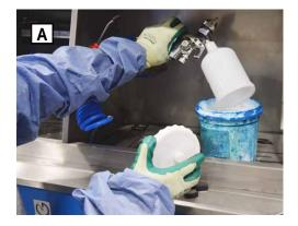
1. Empty the paint cup and remove it from the spray gun (A).
