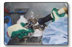
3. If needed, the sink can be used as a soaking tank when using supplied cap (O).
