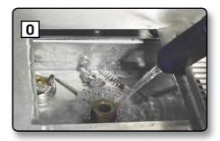
**4.** Dry thoroughly the spray gun, the cup and other disassembled parts using the air blow gun **(P).** No rinsing needed.
