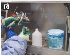
2. Remove the air cap (B) and blow air through the spray gun to remove any residual paint inside (C).
