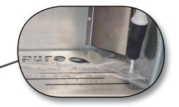
2. Clean the spray gun(s), cup(s), air cap(s) and other disassembled parts using the manual flow-through brush (N).
