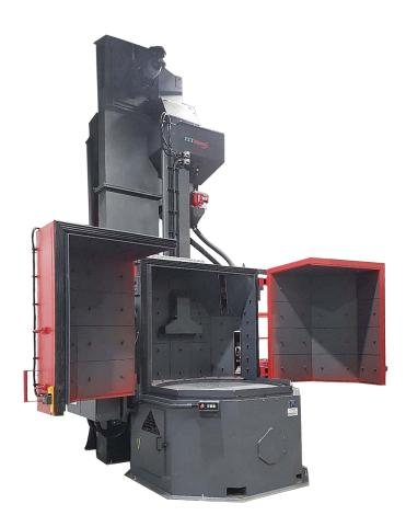
Shot blasting parts of various shapes and dimensions, casts, forged parts, pressed parts, steel and non-ferrous metal parts and parts made from fragile materials, cleaning surface, removing casting sand and filings, consolidating the surface (microhandling), roughing the surface before colouring, etc.
