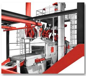
Treated objects are placed on horizontal network conveyor going through the shot blasting machine. In the process of shot blasting the treated objects move through jets of shot blasting agent from turbines, which are installed at different angles with regard to direction of the movement which provides efficient treatment.
