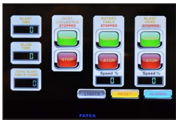
Controlled by HMI
