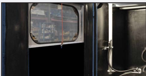
Rubber lining protection inside cabinet and cyclonic separator
