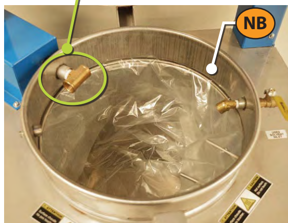
Good installation (bag folded down)
