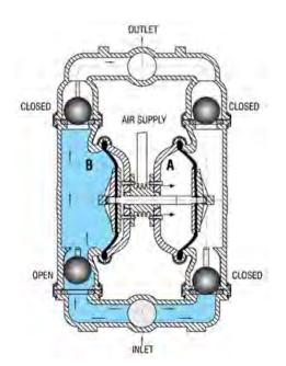
The air-valve directs pressurized air behind the diaphragm on the right, causing the diaphragm on the right to move outward (to the right).
