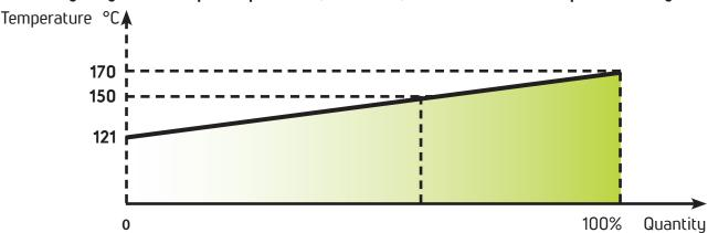
Once a temperature of 150°C (302°F) is reached, which is the critical non–supportable temperature, only 80% of perchloroethylene will be recovered.
