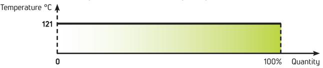
The distillation temperature of a clean solvent remains the same until the process of the whole cycle is complete.
