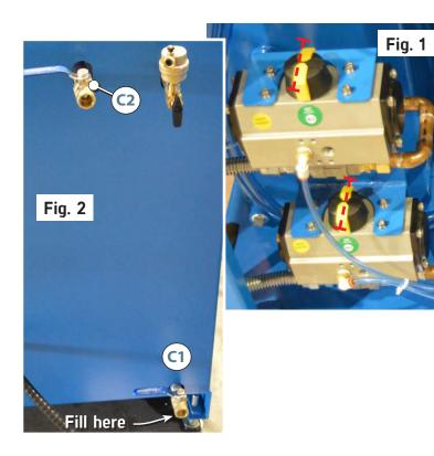
Before you begin, ensure the 2 Rotex valves (Fig. 1) are closed.
