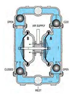
The air-valve directs pressurized air behind the left diaphragm, causing the left diaphragm to move outward (to the left).
