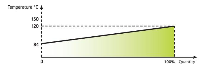
Operating with vacuum condition, 100% of perchloroethylene will be recovered when set at 120°C (248°F) and very far from the critical temperature of 150°C (302°F).
